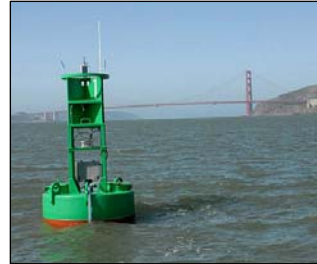
USCG navigational buoy used to mount the communications gateway consisting of a hydrophone below, a small computer and wireless internet.
