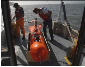
The "Stablemoor" buoy being readied for deployment in the San Francisco Bay. The buoy houses the ADCP, acoustic release and acoustic modem.
