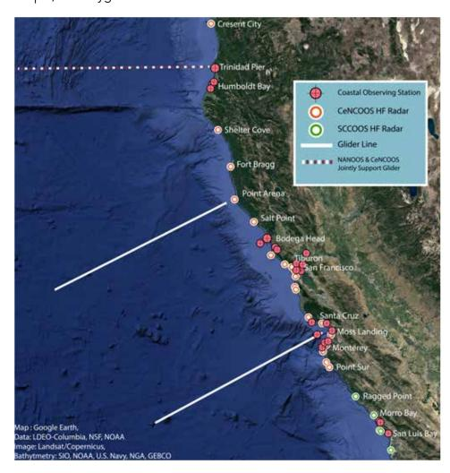
CeNCOOS connects users to data from 26 high-frequency radar (HFR) stations, more than two dozen coastal stations and moorings, autonomous vehicles including gliders, animal telemetry, ship surveys, and many other platforms and sensors.
